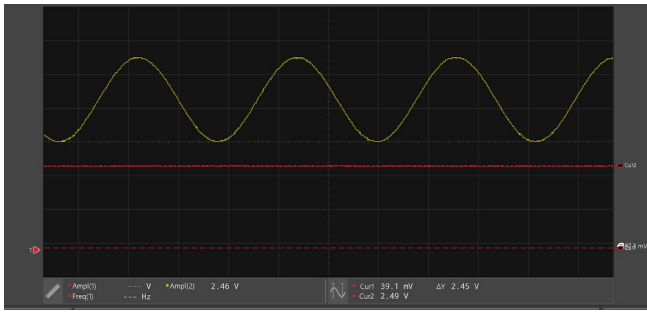
Figure 11: V_g High Pass MOSFET Voltage with 2.5 Volt Sinusoid Signal at 1500 Hz
